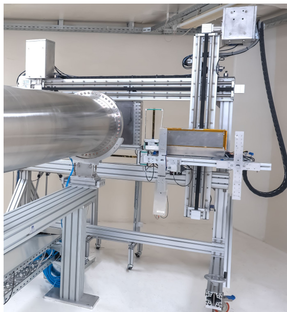
Figure 6. The robotic table at the target region shows several movable test stations.
